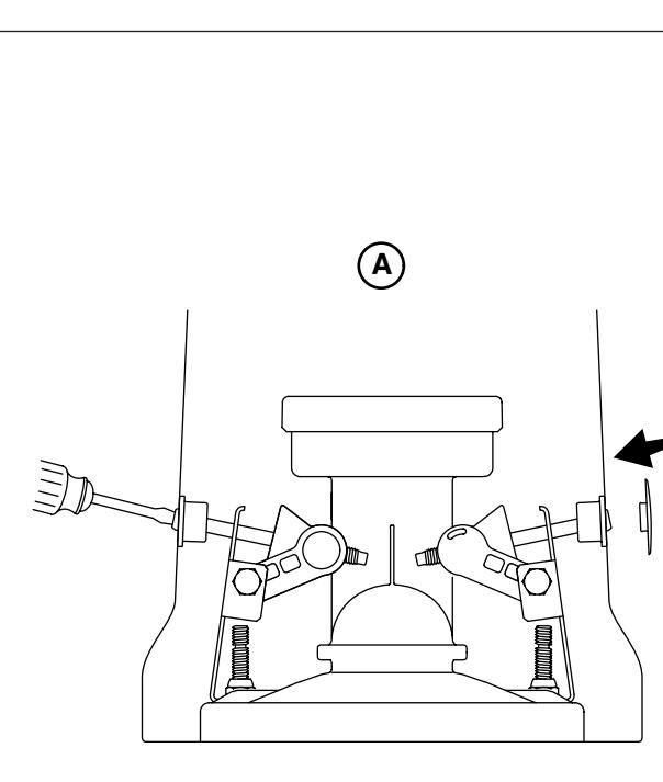
17A. With the rod nuts  $7/8"$  (22 mm) from the end of the push button rods, thread the push button rods into the button housing.
